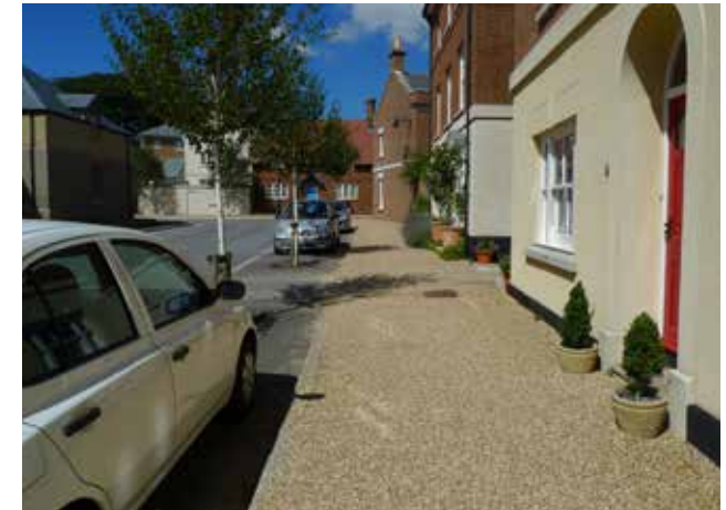
Figure 26: Example of on-street parking with parking bays and street trees to mitigate the impact of the cars on the streetscape, Poundbury, Dorset.
