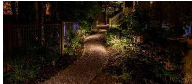
Figure 32: Example of path lighting, use of flow fixtures which direct illumination downwards and outward.
