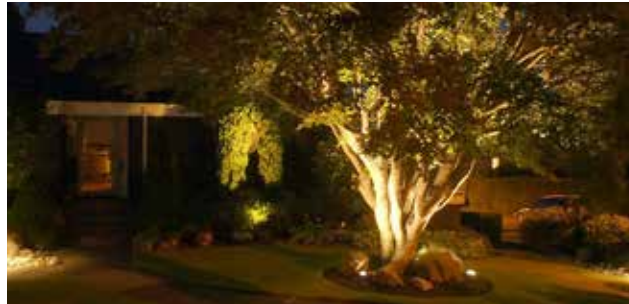
Figure 31: Example of up-lighting, light is focused on an object or tree from a low fixed location.
